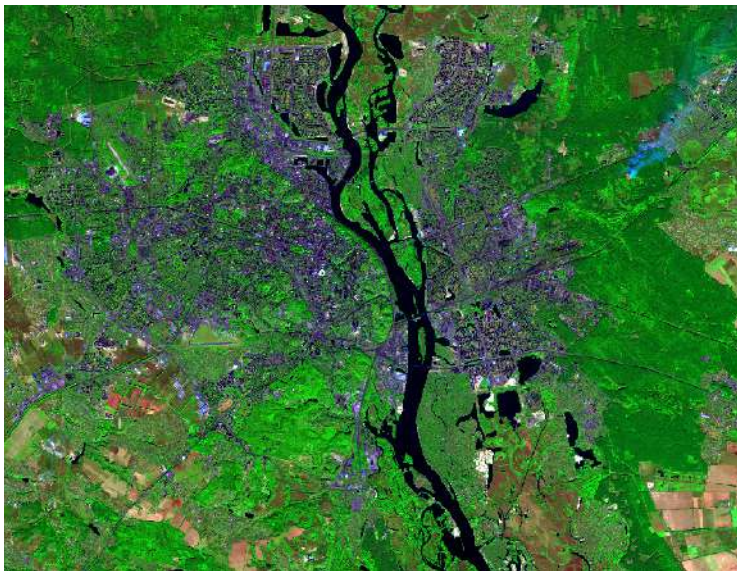
Fig. 1.142. The resulting color image of Kyiv (combination of bands: B12, B8, B2)
