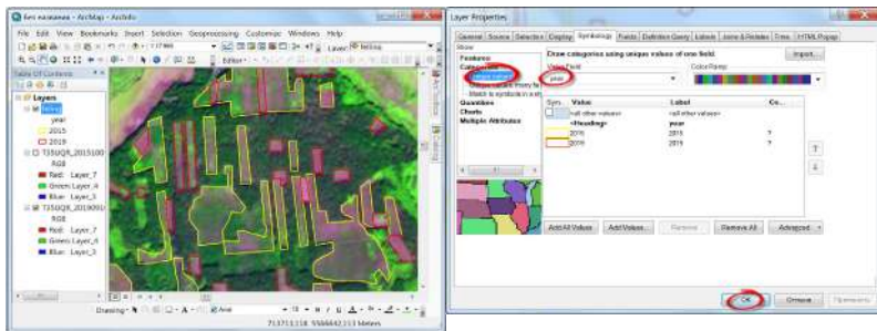
Fig. 2.24. Selecting display styles for the felling vector by category and the code of felling year, respectively
