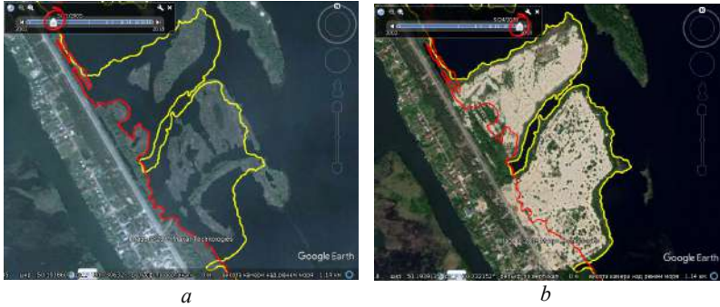
Fig. 2.66. Comparing the views of the islands using the Show historical imagery tool. The red color of the shoreline for 2018 and the yellow for 2005 are superimposed on the image: 2005 (a), 2018 (b)
