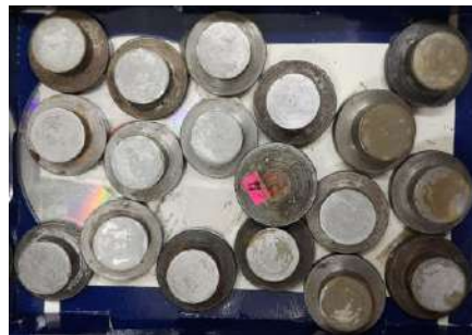
Fig. 4. Glued steel tear-off plates for adhesive strength determination
