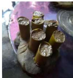
Fig. 3. Cylindrical samples for compressive strength tests
