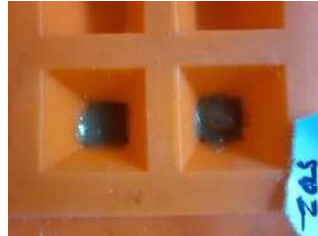
Fig. 5. Sample tablets for testing in in aggressive fluids
