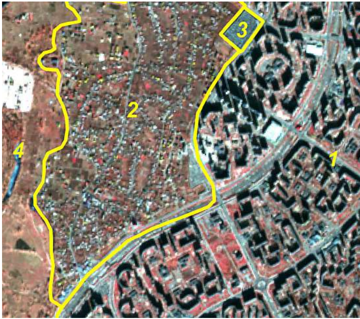
Fig. 3.1. Example of building system interpretation (1 — town area with blocks of flats; 2 — single- and two-storey buildings in the suburbs; 3 — garages, industrial areas; 4 — undeveloped meadowland)
