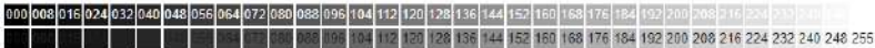
Fig. 1.4. Example of color gradation in the 8-bit image, where 1 byte of information contains 256 colors (e.g. shades of gray). Black represents a digital number of “0” and white represents a digital number of “255” [3]
