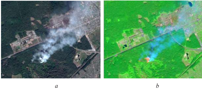
Fig. 1.106. Place of fire in the satellite image collected by Sentinel 2: a combination of B04, B03, B02 bands (a), a combination of B12, B08, B02 bands (b)
