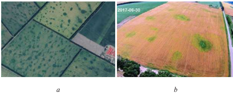
Fig. 2.89. Manifestations of loess subsidence in Baryshivskiy District in the Google Earth Pro satellite image (a) and example of wheat yield reduction and intensification of weed overgrowth on aerial photo (b)
