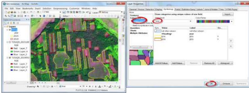
Fig. 2.24. Selecting display styles for the felling vector by category and the code of felling year, respectively
